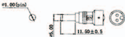
4. \varnothing 1.00(\text{pin}) \times 5.00 \times 11.5 \pm 0.5 mm "I" type , yellow
