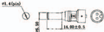
5. \varnothing 1.40(\text{pin}) \times 6.50 \times 14 \pm 0.5 mm "I" type , black
