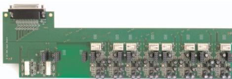
Extension Modul for 8 Inputs, Electronically Balanced
